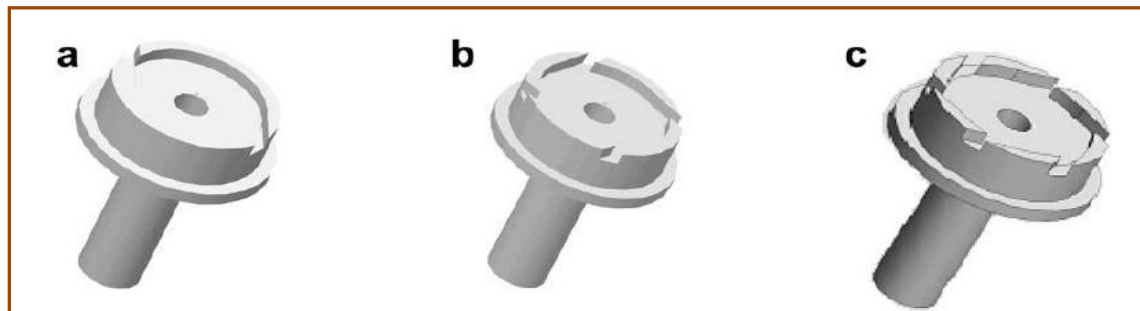
Fig. 11 Nozzles used in experiments: (a) 2 nozzle, (b) 4 nozzle, and (c) 6 nozzle
