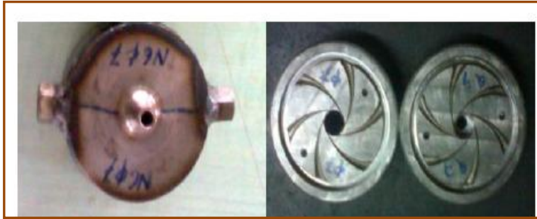
Fig. 7. Inlet cap (cold end) and Geometry for convergent nozzle
